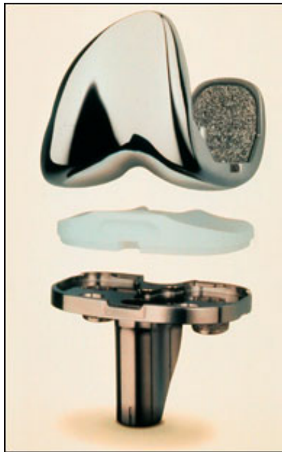
Figure 3B shows the components of a typical total knee replacement. The white polyethylene locks into the bottom piece, which is called the tibial tray. The top part caps the prepared end of the femur. Actual movement of the artificial knee takes place between the top portion and the polyethylene layer.
